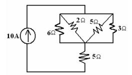
b) Find the all branch currents and voltage across all the resisters in the below circuit diagram.
