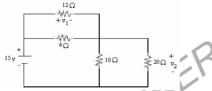
b) Calculate  $R_{\text{eq}}$  in the below circuit diagram.
